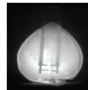
Flame propagation and venting of a flammable event in a 5-L glass sphere Venting was initially seen at 45 ms
